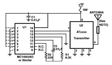
NOTE: This matching component is required only for antennas that are not 50 ohms. It is typically a chip inductor to match to stub antennas shorter than 1/4 wavelength. For very low radiated field—strength applications, a resistor can also be used.
